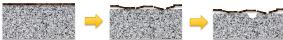
Fig. 2. Using the concept of scaling tendency to describe pit initiation in CO<sub>2</sub> environments by undermining effect.
